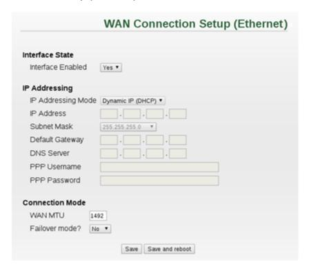
For many setups the default addressing mode of 'Dynamic IP (DHCP)' will be suitable, but the device allows configuration of 'Static IP' and 'PPPoE' options if needed.
