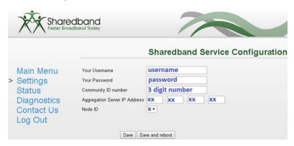
The details required for this screen are those generated when creating the user on the Sharedband NOC. The only value which differs is the 'Node ID' (1 - 8) depending on the Router number of your WAN Ethernet connection.
