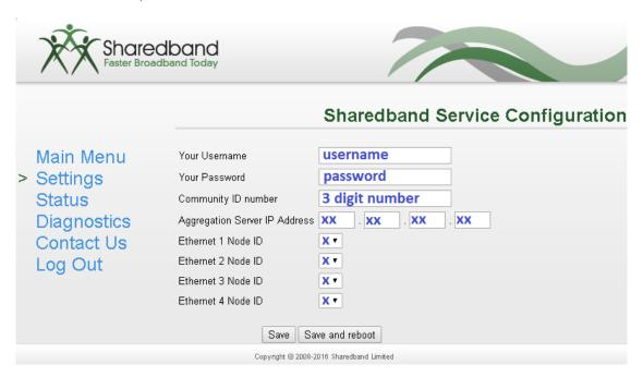
The details required for this screen are those generated when creating the user on the Sharedband NOC. For typical WR1043ND MultiWan deployments with a single device, leave the '**Node ID**' values for the four interfaces at the defaults of 1, 2, 3 and 4.
