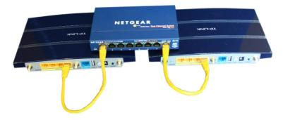
b) However you can connect the Sharedband routers together with an Ethernet cable (daisy chained)
