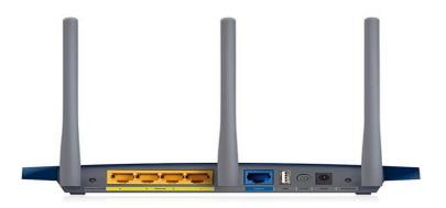
**Step 3:** Log onto the Web interface of the router (default address <u>http://192.168.0.1</u>). The default login is '**admin**' and password '**admin**'.
