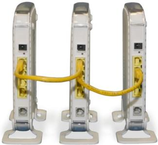
Or plug both Sharedband Routers together with an Ethernet cable.
